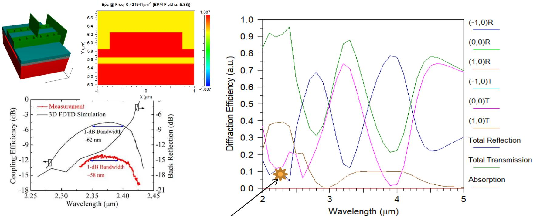
The simulated back-reflection is lower than -10 dB from the wavelength of 2.26 μm to the wavelength of 2.4 μm.
